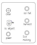
You will find the control panel at the back of the machine. This panel includes one button, one adjustable screw and four indicator LEDs.
